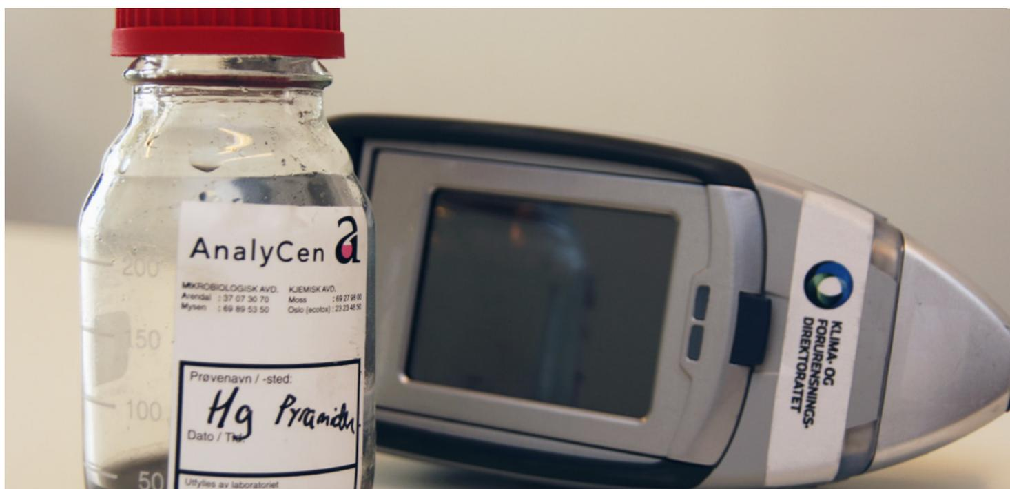
Handheld X-ray fluorescence (XRF) analyser for rapid measurements of about 30 elements. XRF can be used to measure the content of heavy metals in alloys, plastics, wood, stone, soil and painted surfaces, and is increasingly being used in controls of ordinary consumer products such as toys and electronic goods.
