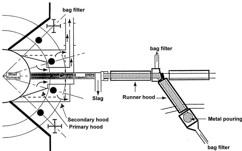
Figure 9.17: Hooding system for a blast furnace
