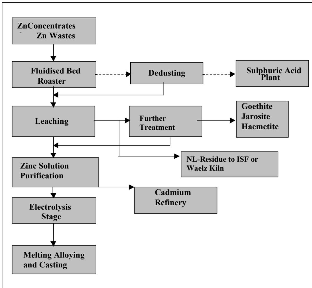
Figure 5.5: Diagram of the zinc hydrometallurgical process
