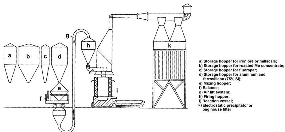
**Figure 9.8: Metallo-thermic firing arrangement**
