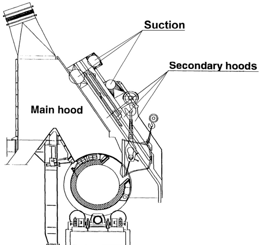
Figure 2.27: Secondary hooding system for a converter
