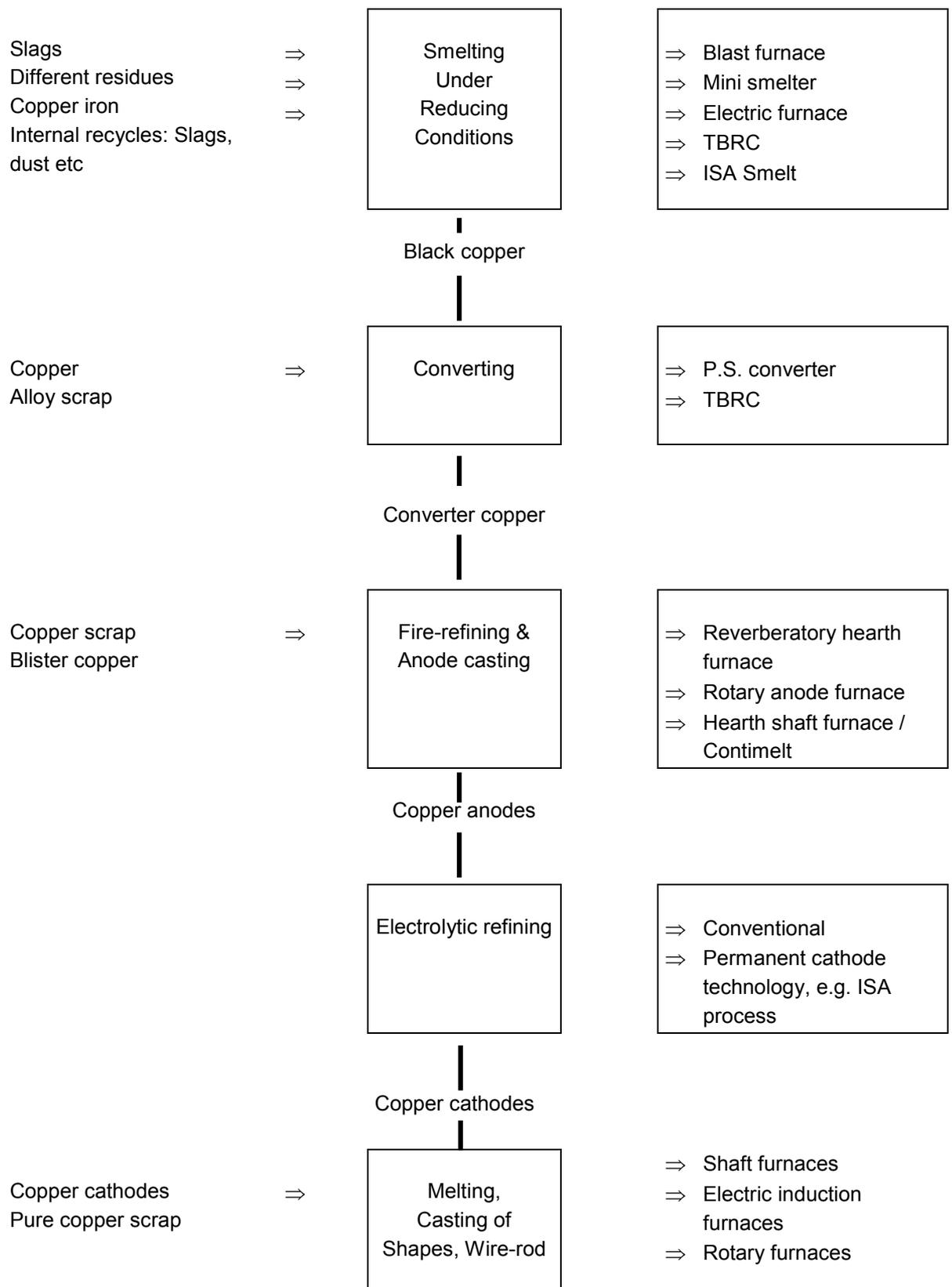
Figure 3.3: Generic flow sheet for secondary copper production
