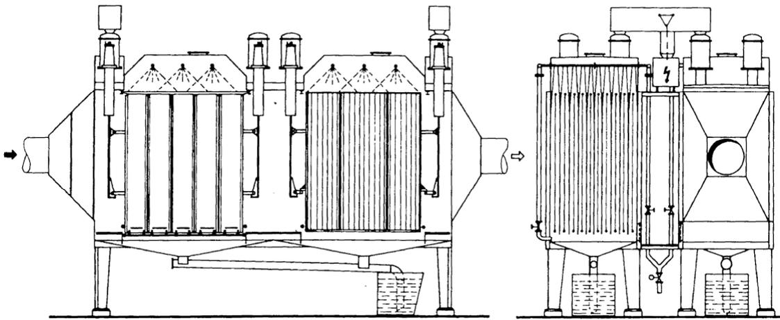
**Figure 2.31: Wet electrostatic precipitator**
