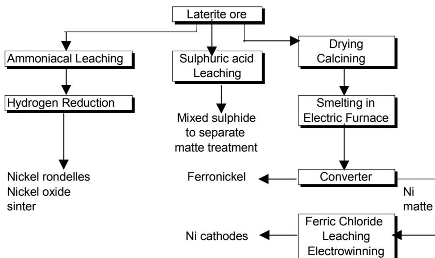
**Figure 11.1: Generic flow sheet for nickel production from Laterite ores**
