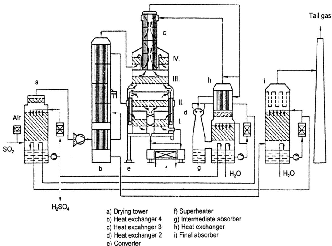
Figure 2.37: A Typical Double Absorption Sulphuric Acid Plant
