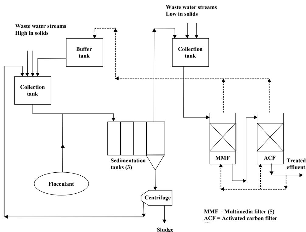
**Figure 10.11: Treatment plant for cleaning dioxin and chlorinated hydrocarbon contaminated wastewater**
