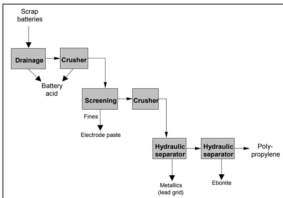
**Figure 5.2: Outline of a typical battery recovery process**
