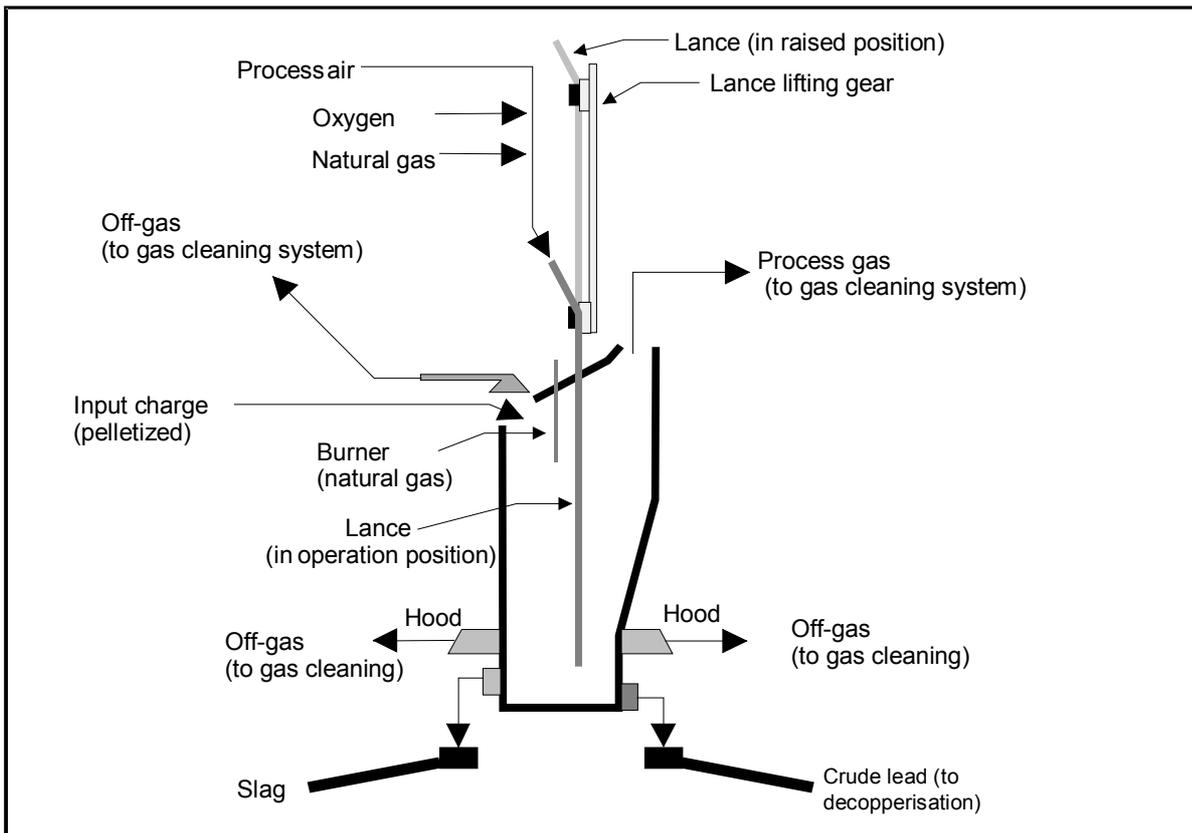
**Figure 2.9: The Ausmelt/ISA Smelt process**
