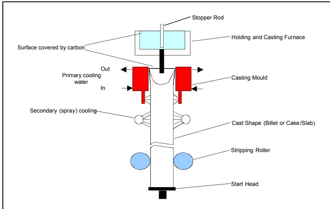
**Figure 3.7: Principle of continuous or semi-continuous casting**
