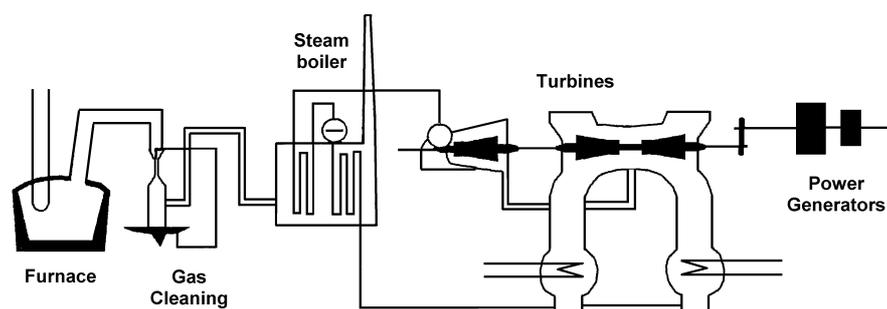
Figure 9.18: Direct use of the CO gas for the production of electrical energy
