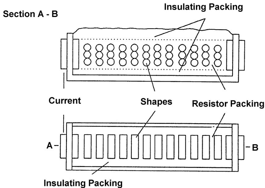
**Figure 12.5: Acheson graphitising furnace**
