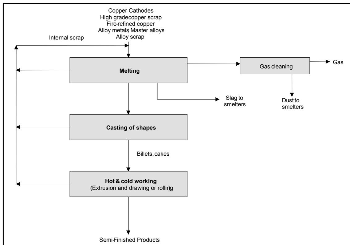
**Figure 3.6: General flow-sheet of semi-finished product fabrication**
