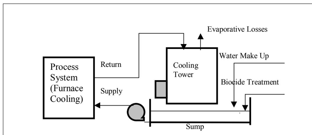
**Figure 2.40: Example of a Cooling Water Re-circulation System**
