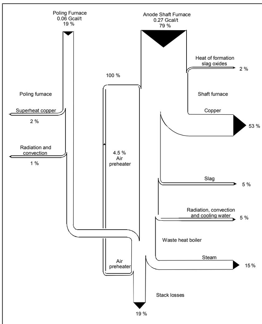
**Figure 2.43: Energy balance of the Contimelt process**
