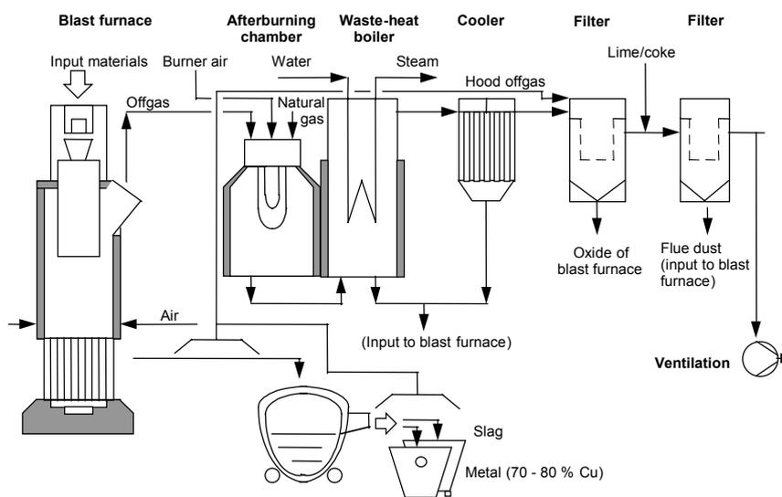
**Figure 3.14: General arrangement of an afterburner system**
