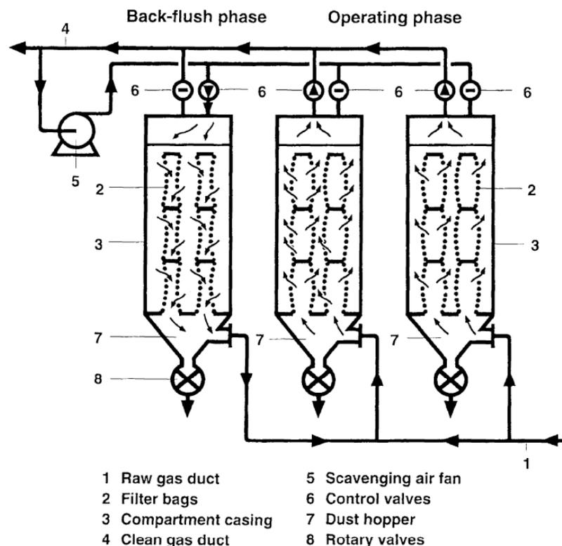
Figure 2.33: General arrangement of a fabric filter (with one compartment in the cleaning cycle) [tm 198, Lurgi 1999]
