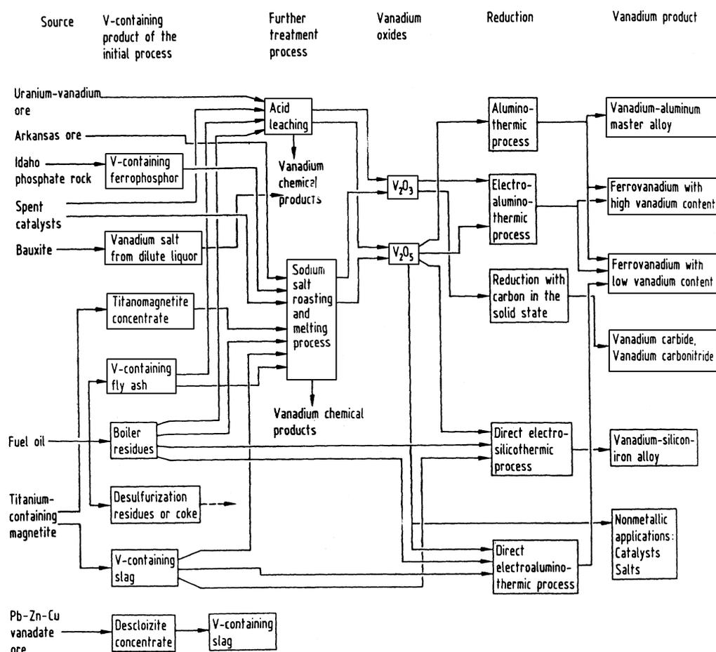
Figure 8.6: Production of vanadium pentoxide and vanadium metal [tm 008, HMIP 1993]
