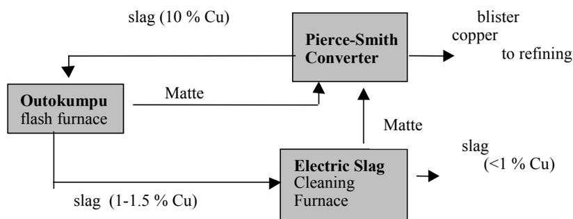
**Figure 2.41: Electric furnace cleaning of copper slags**
