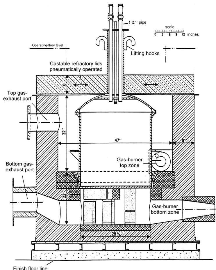
**Figure 8.7: Reaction vessel of the titanium production using the Kroll process**
