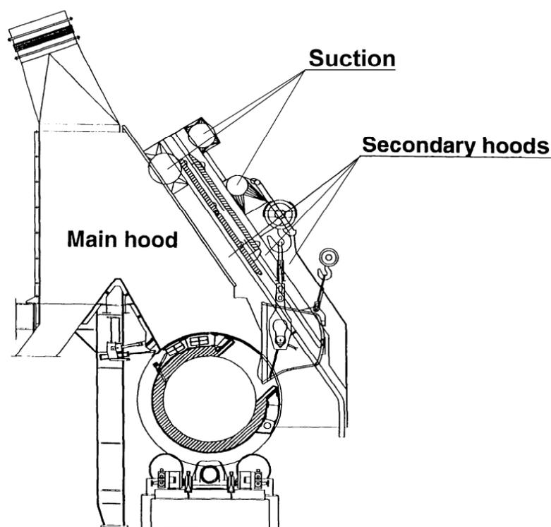
Figure 3.13: Targeted secondary fume capture system
