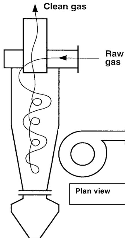
**Figure 2.32: Arrangement of a cyclone**
