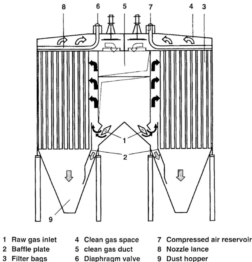
Figure 2.34: Reverse pulsed jet cleaning system [tm 198, Lurgi 1999]
