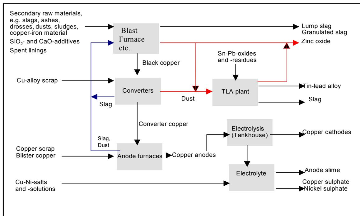
**Figure 3.11: Example of an Input–Output diagram from a secondary copper production site with a tin/lead recovery process**
