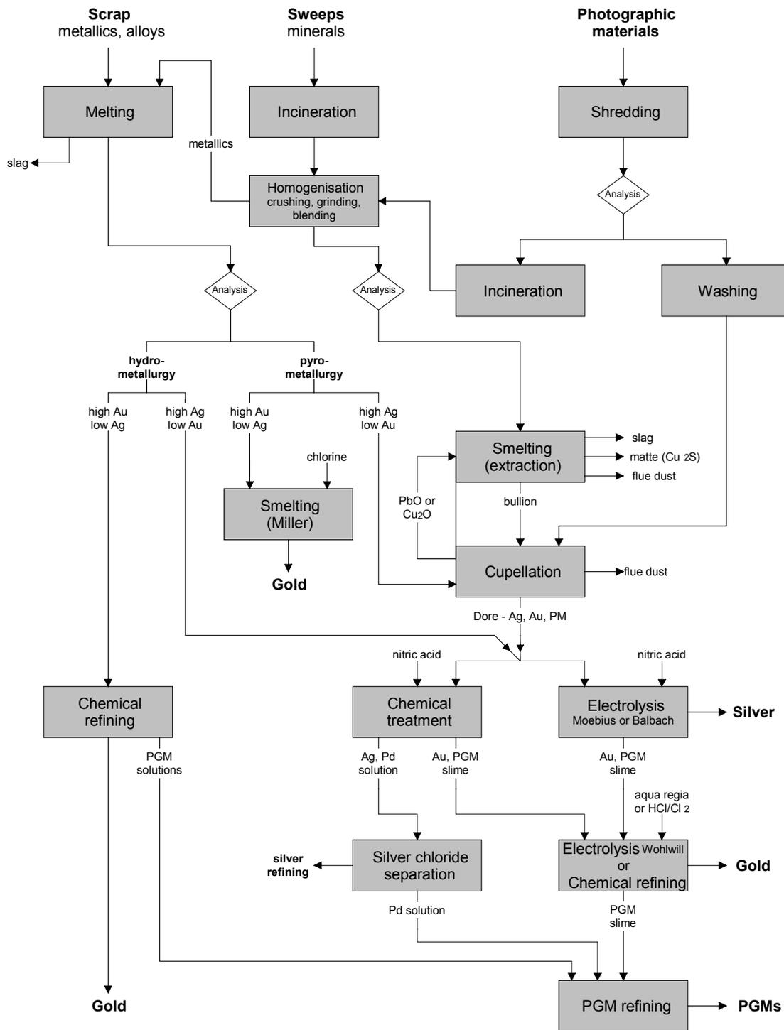
Figure 6.1: General flow-sheet for precious metal recovery
