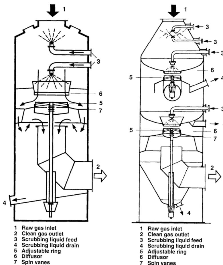
**Figure 2.35: Radial flow scrubber**
