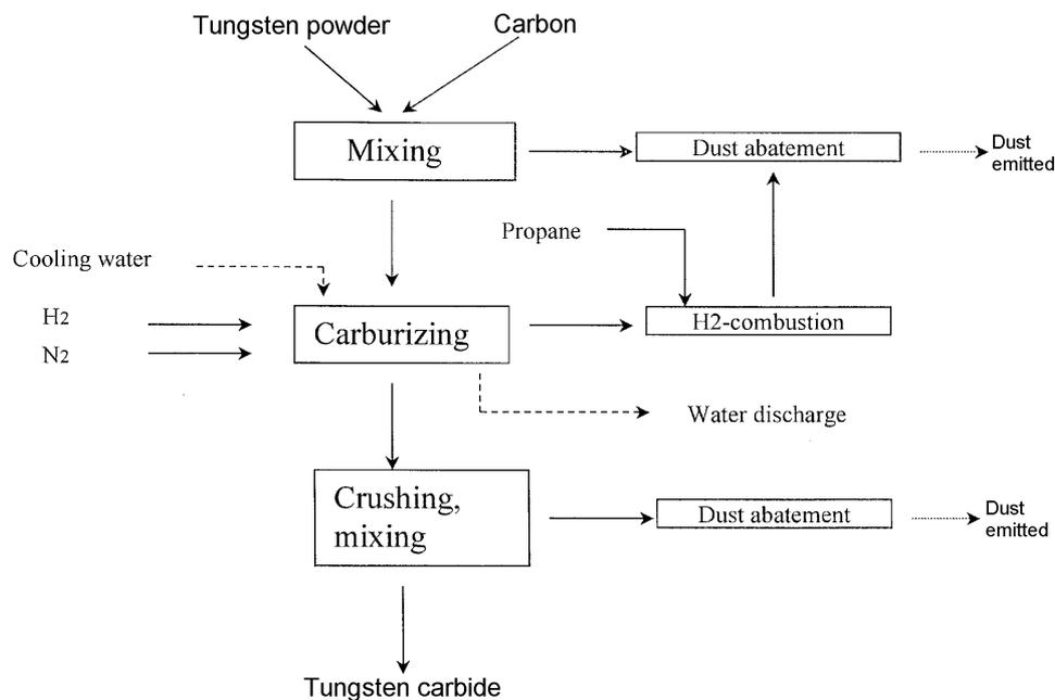
**Figure 8.5: Production of tungsten carbide**
