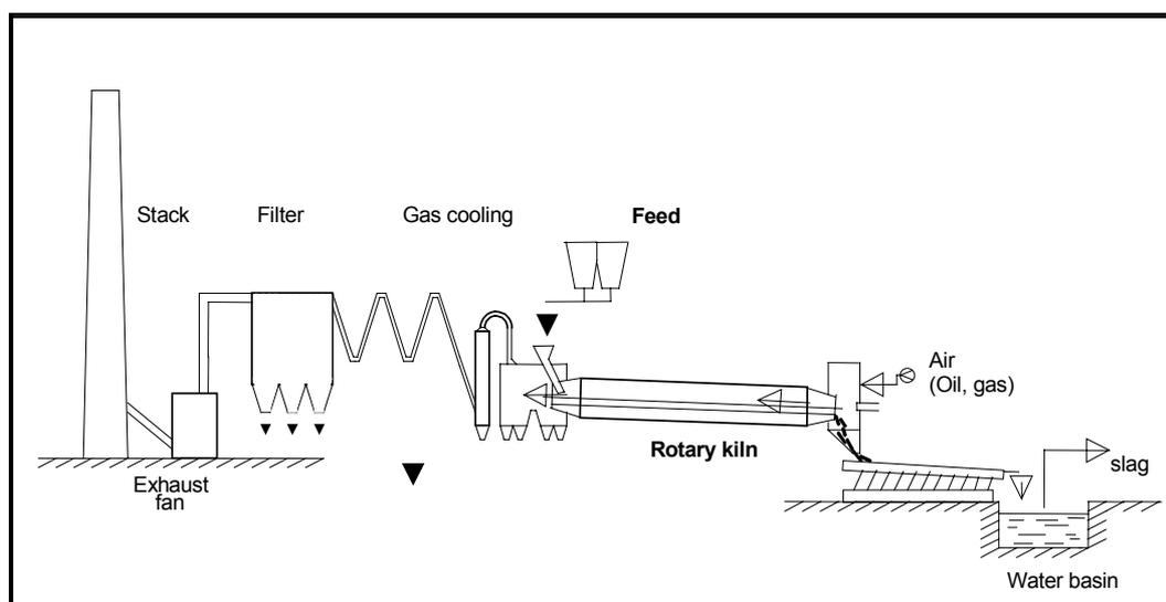
**Figure 2.1: Rotary kiln**
