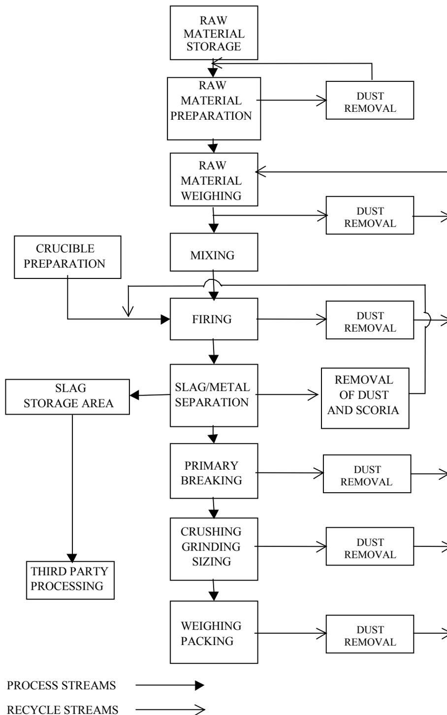
Figure 9.9: Production of ferro-molybdenum by a metallo-thermic reduction
