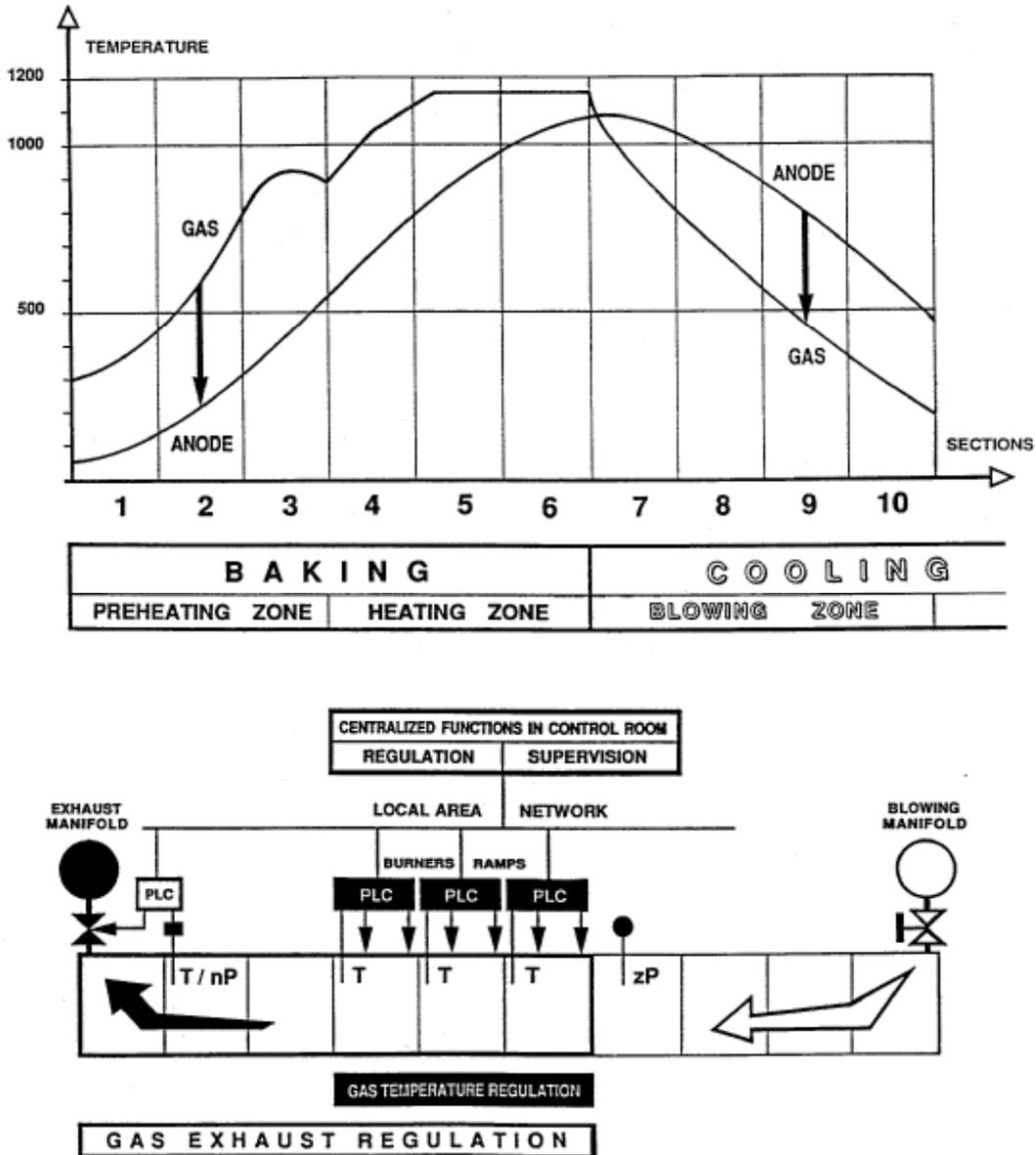
Figure 12.3: Temperature profile during the baking of anodes
