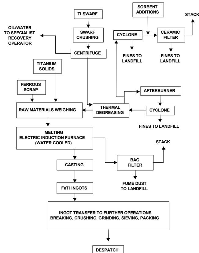
Figure 9.10: Flow diagram of the ferro-titanium production
