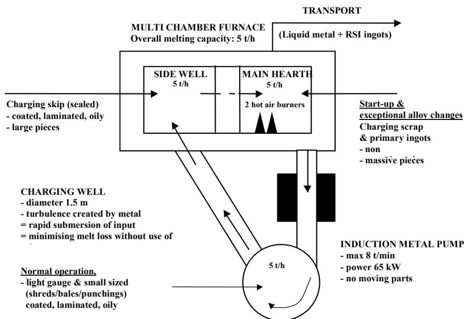
Figure 4.6: An example of a pumped metal system
