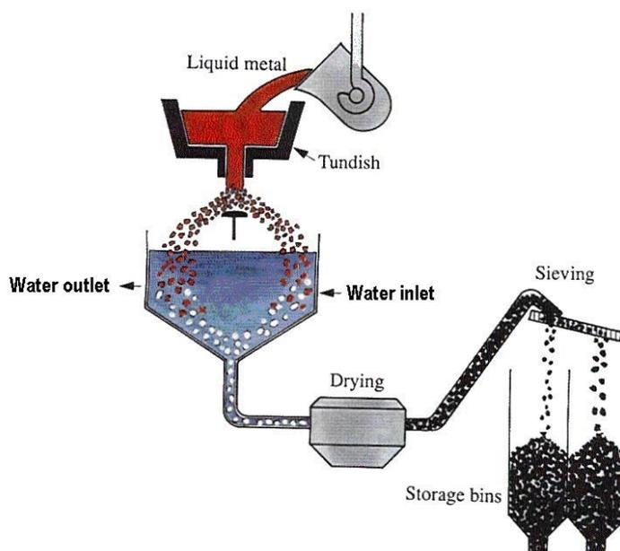
**Figure 2.39: Granulation of molten metal**
