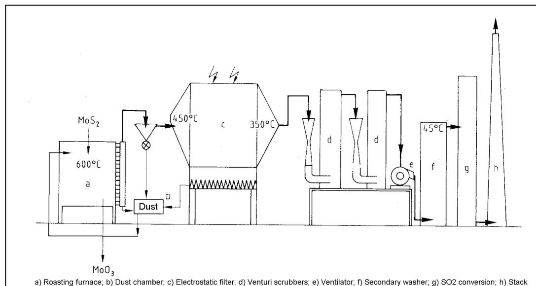
**Figure 8.11: The recovery of rhenium from the flue gases in the roasting of molybdenite**
