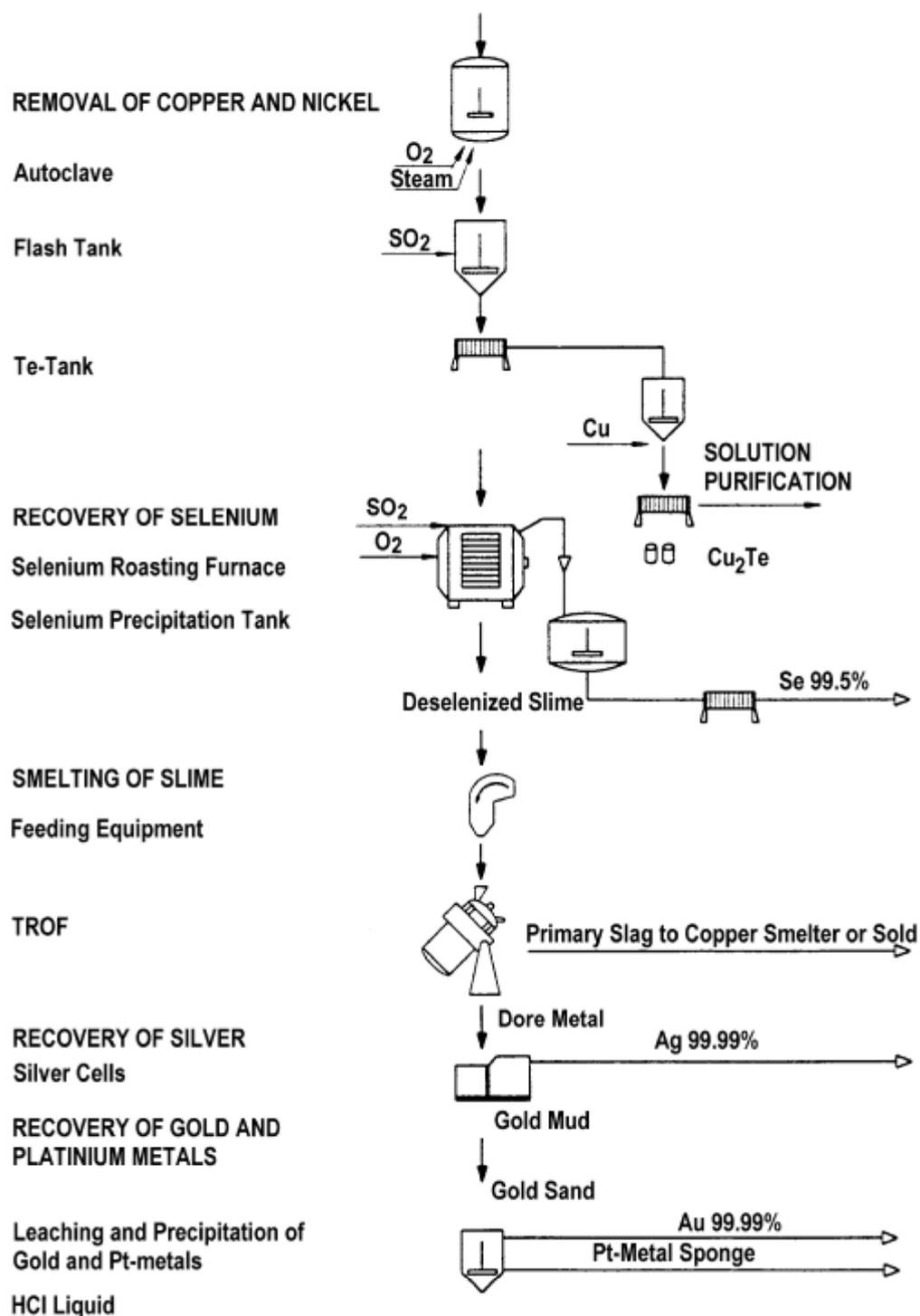
Figure 6.2: Example flow-sheet for anode slime treatment
