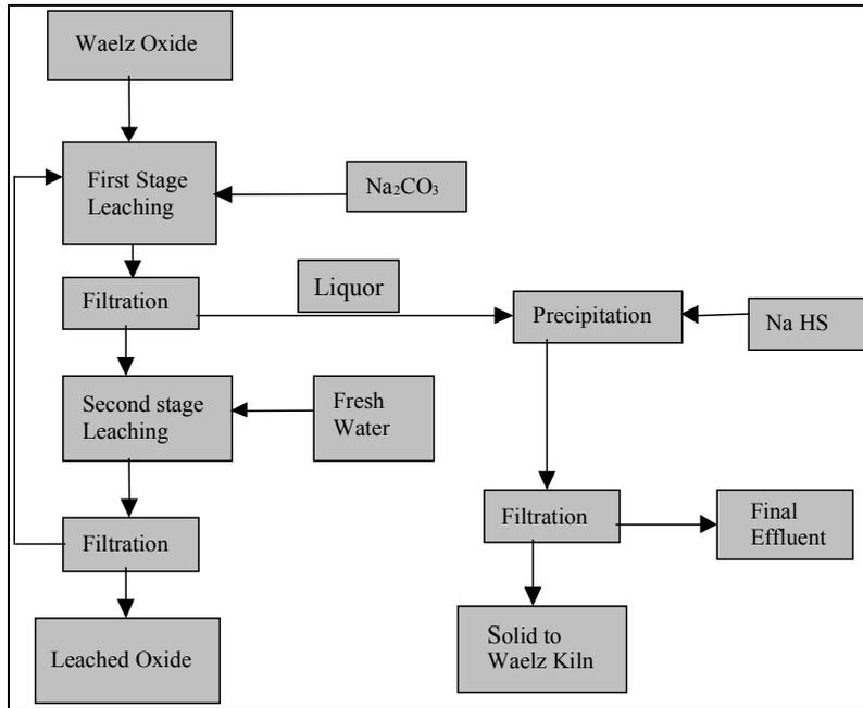
Figure 5.11: Diagram of a Waelz oxide washing circuit
