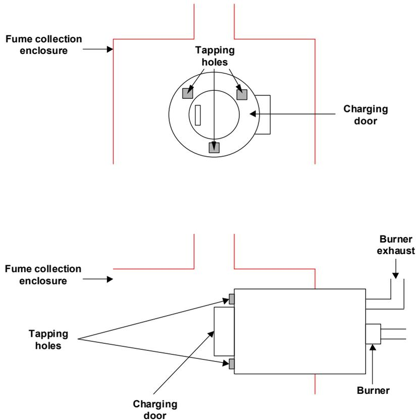
**Figure 6.5: Co-incident fume capture system**
