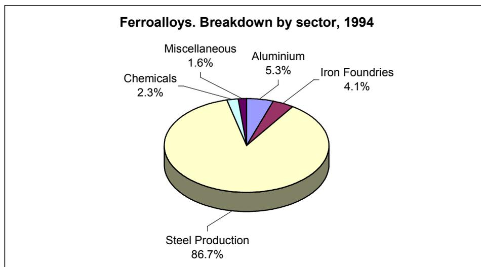
**Figure 1.9: Use of ferro-alloys in different industrial sectors in 1994**
