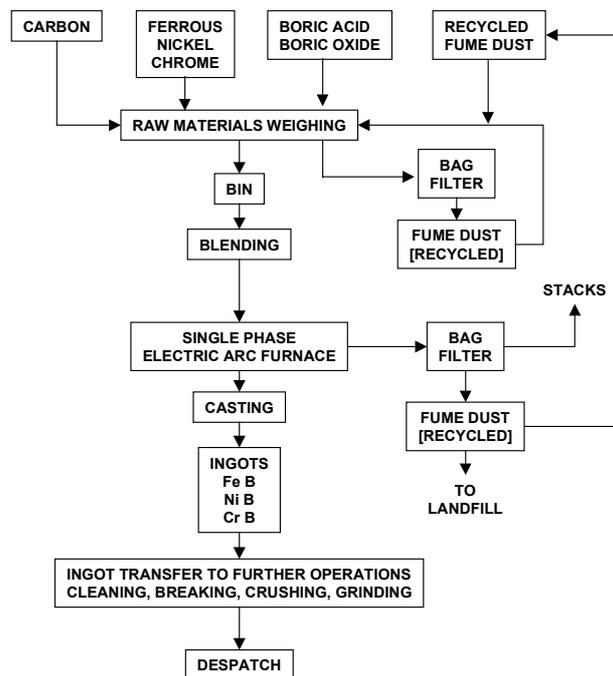
Figure 9.11: Process for ferro-boron and boron –alloy production
