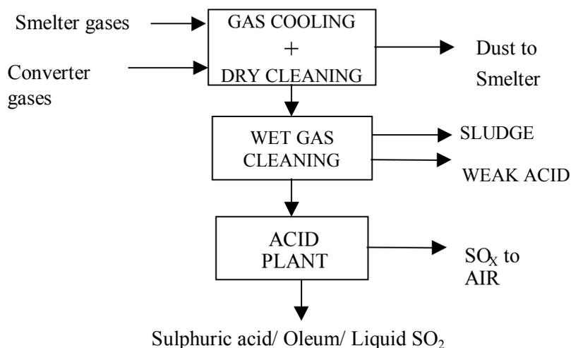
**Figure 3.9: Treatment of smelter and converter gases**
