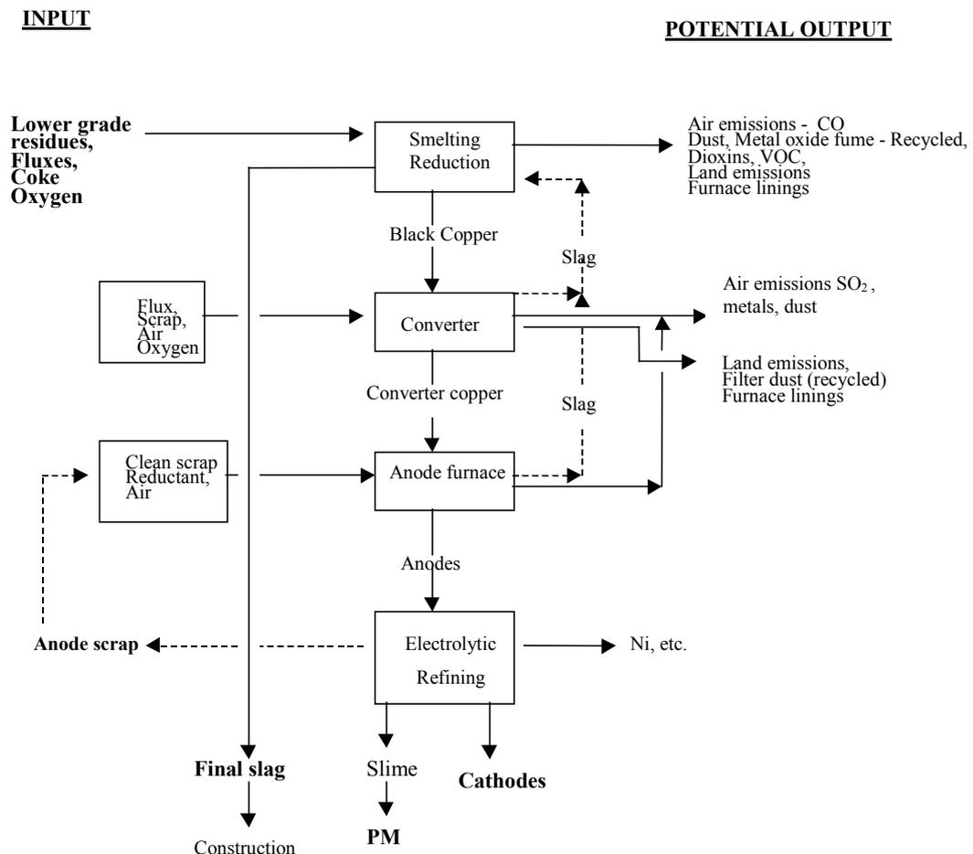
Figure 3.10: Generic input-output diagram for secondary copper smelting
