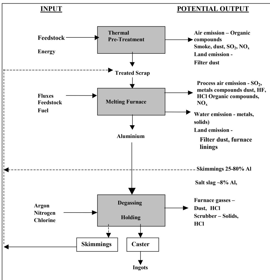
**Figure 4.5: Input and output from secondary aluminium production**
