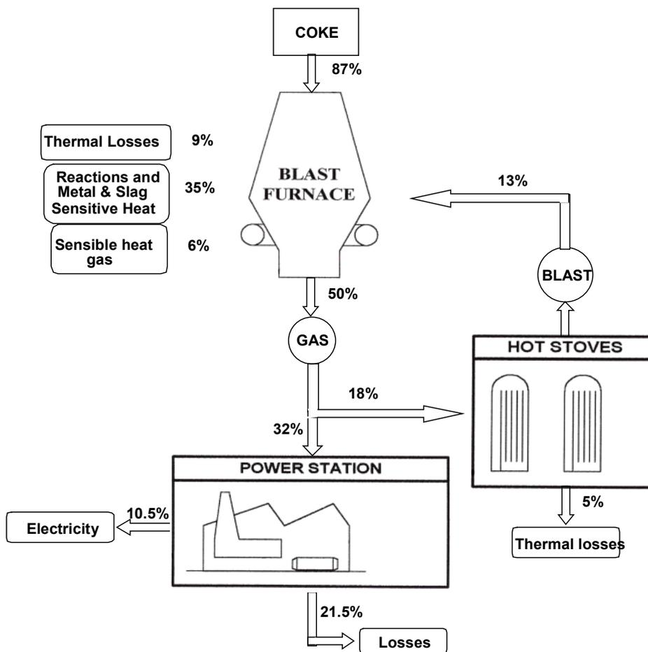
**Figure 9.20: Energy recovery system for a blast furnace**
