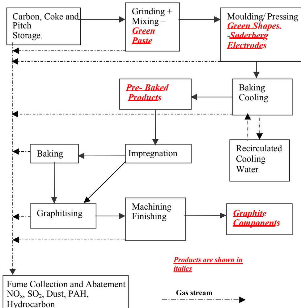
Figure 12.7: Generic emission diagram of the processes used
