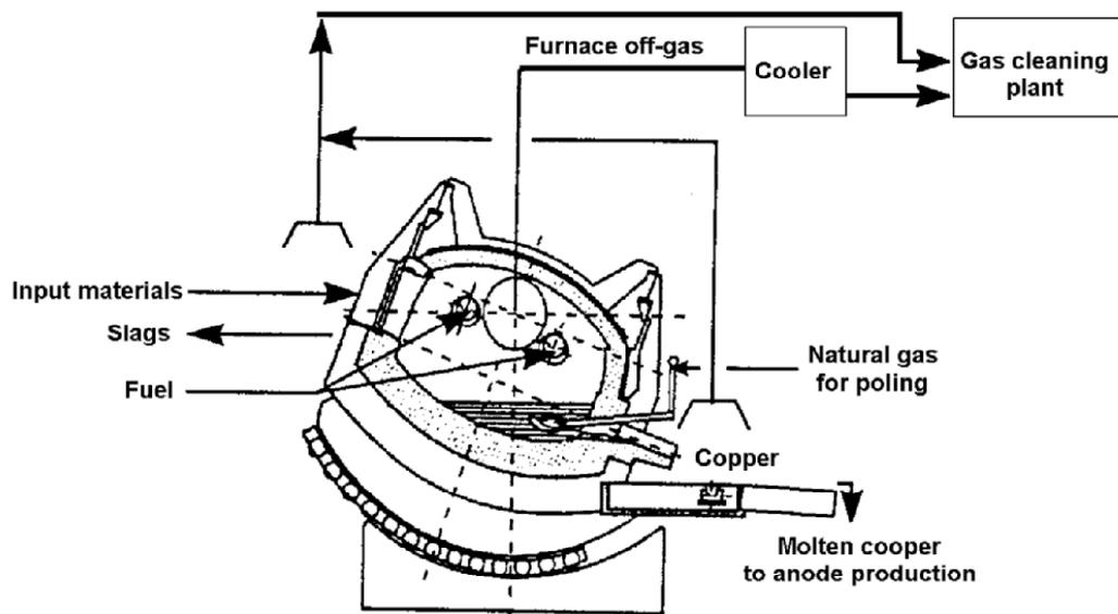
**Figure 2.4: An example of a tilting reverberatory hearth furnace used for secondary materials [tm 124, DFU Cu 1999; tm 226, VDI 2102 1999]**
