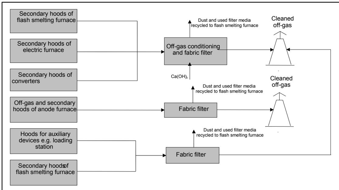
**Figure 2.28: Outline secondary fume collection system for a primary copper process [tm 124, DFIU Cu 1999]**
