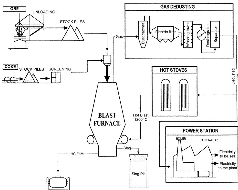
**Figure 9.4: Production of HC FeMn in a blast furnace**
