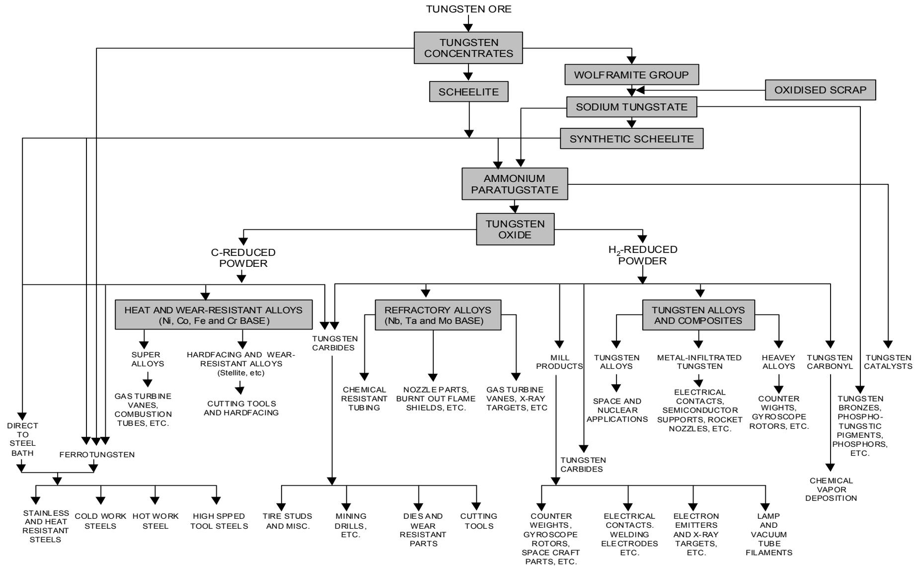
Figure 8.3: Tungsten flow-sheet
