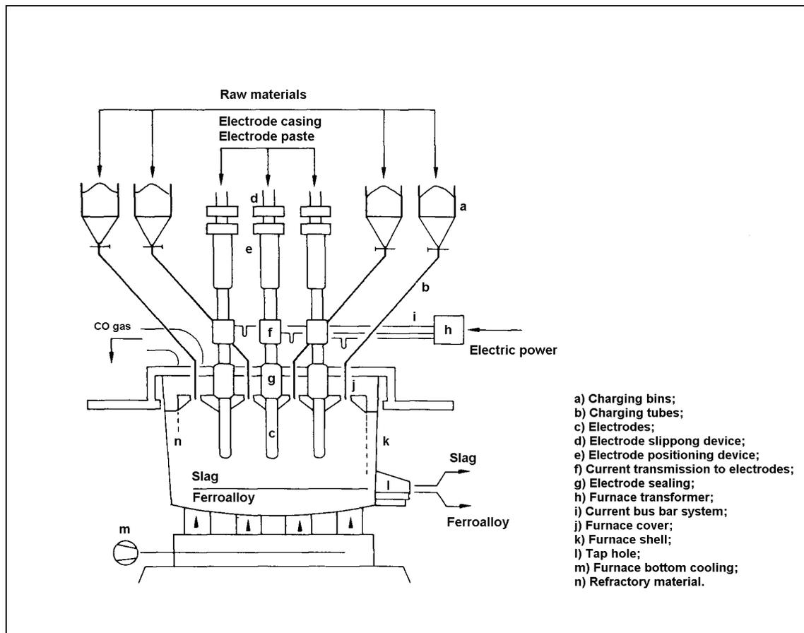
**Figure 9.5: Closed electric arc ferro-manganese furnace operating Söderberg electrodes**
