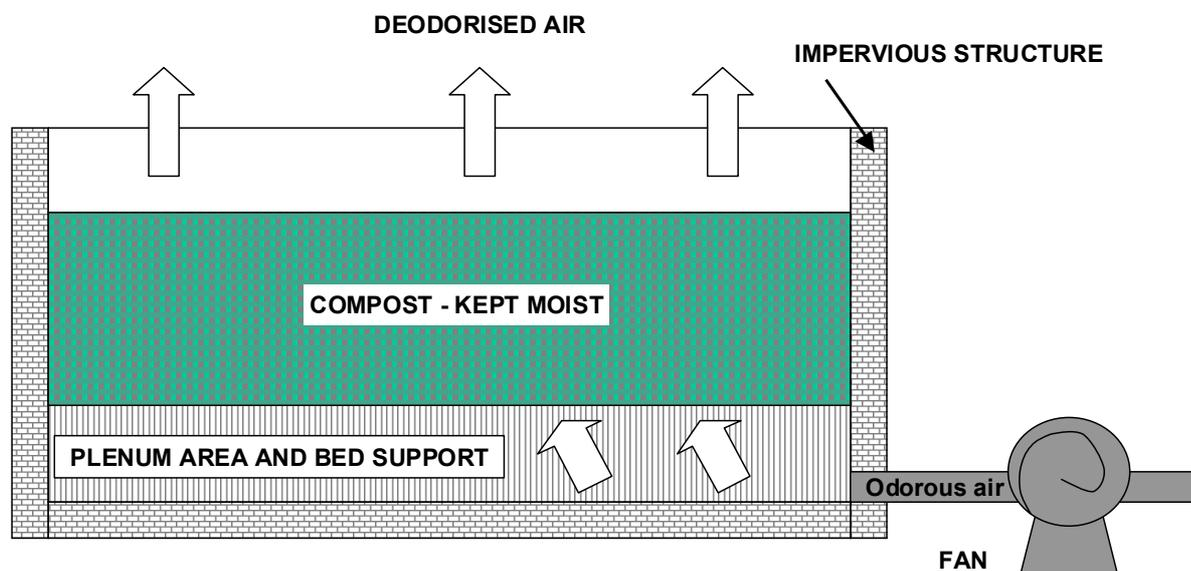
Figure 12.9: Example of a Bio-filter
