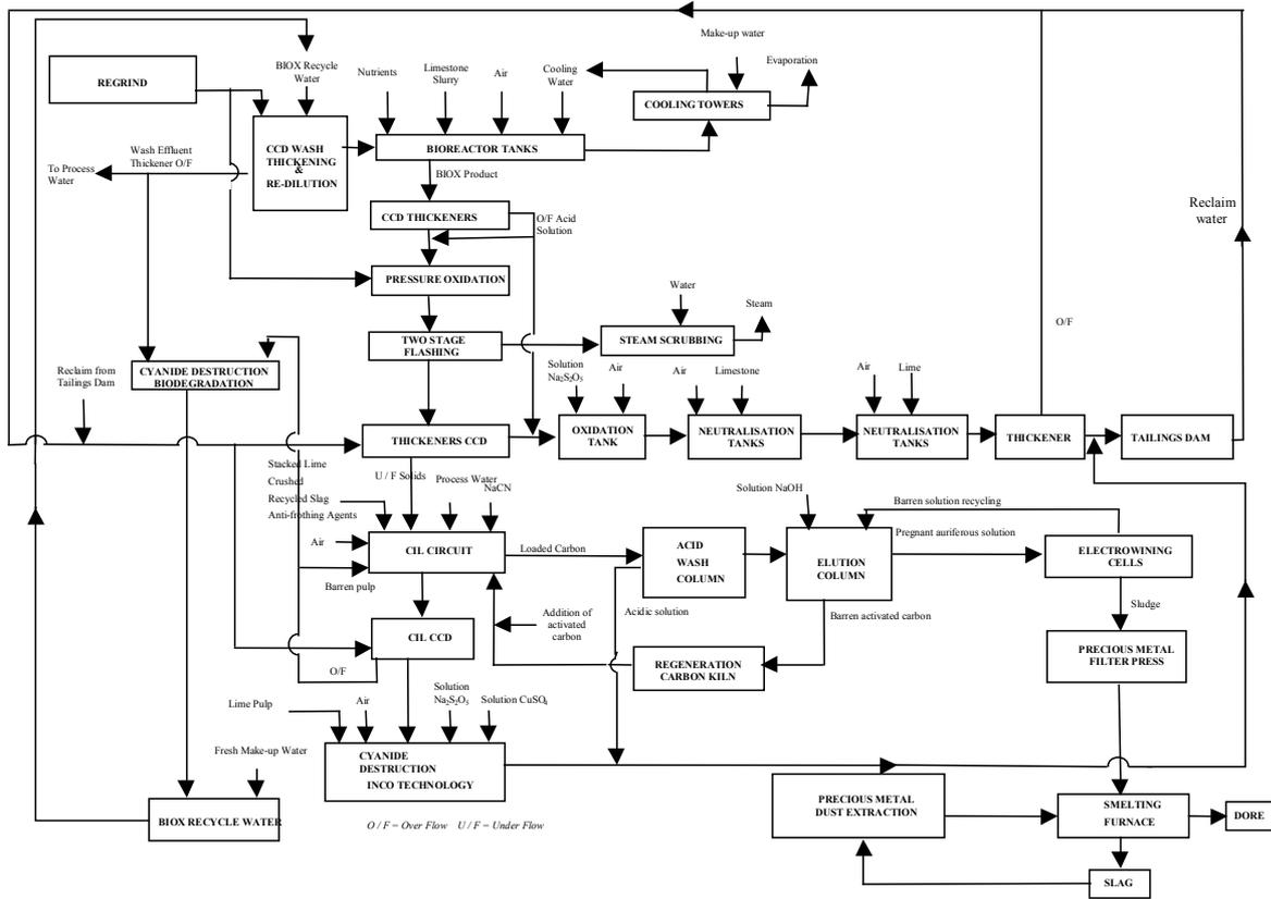
Figure 6.7: Metallurgical process flow-sheet
