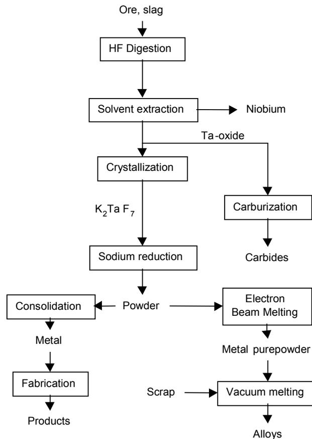
Figure 8.9: Production of pure tantalum metal powder
