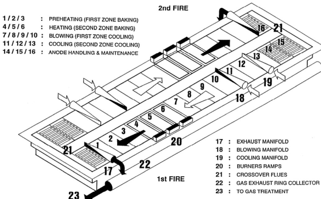
Figure 12.2: General views of an open baking furnace for anodes
