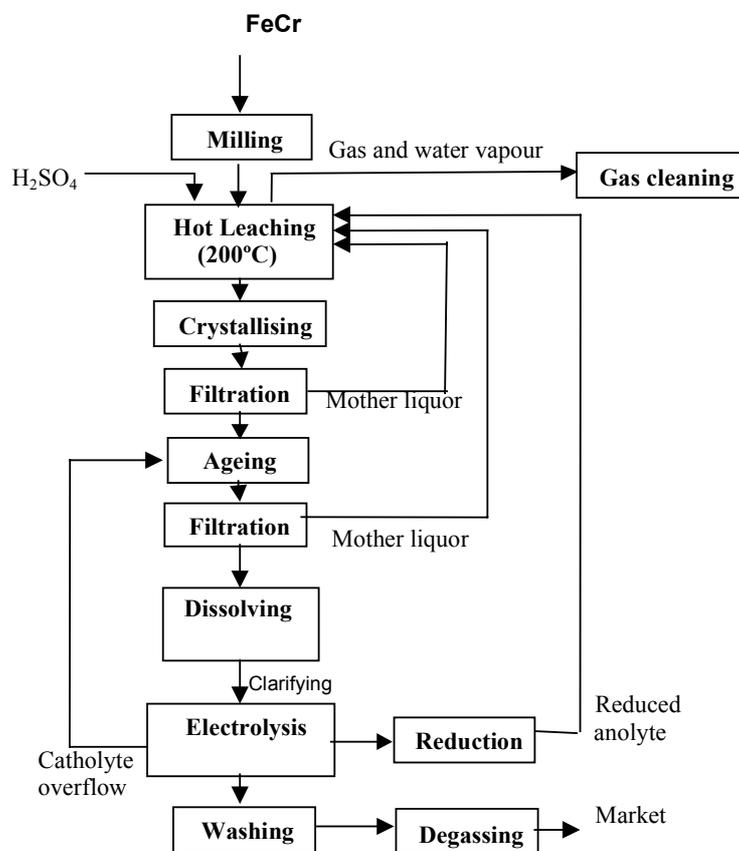
**Figure 8.2: Production of chromium metal by electrolysis**
