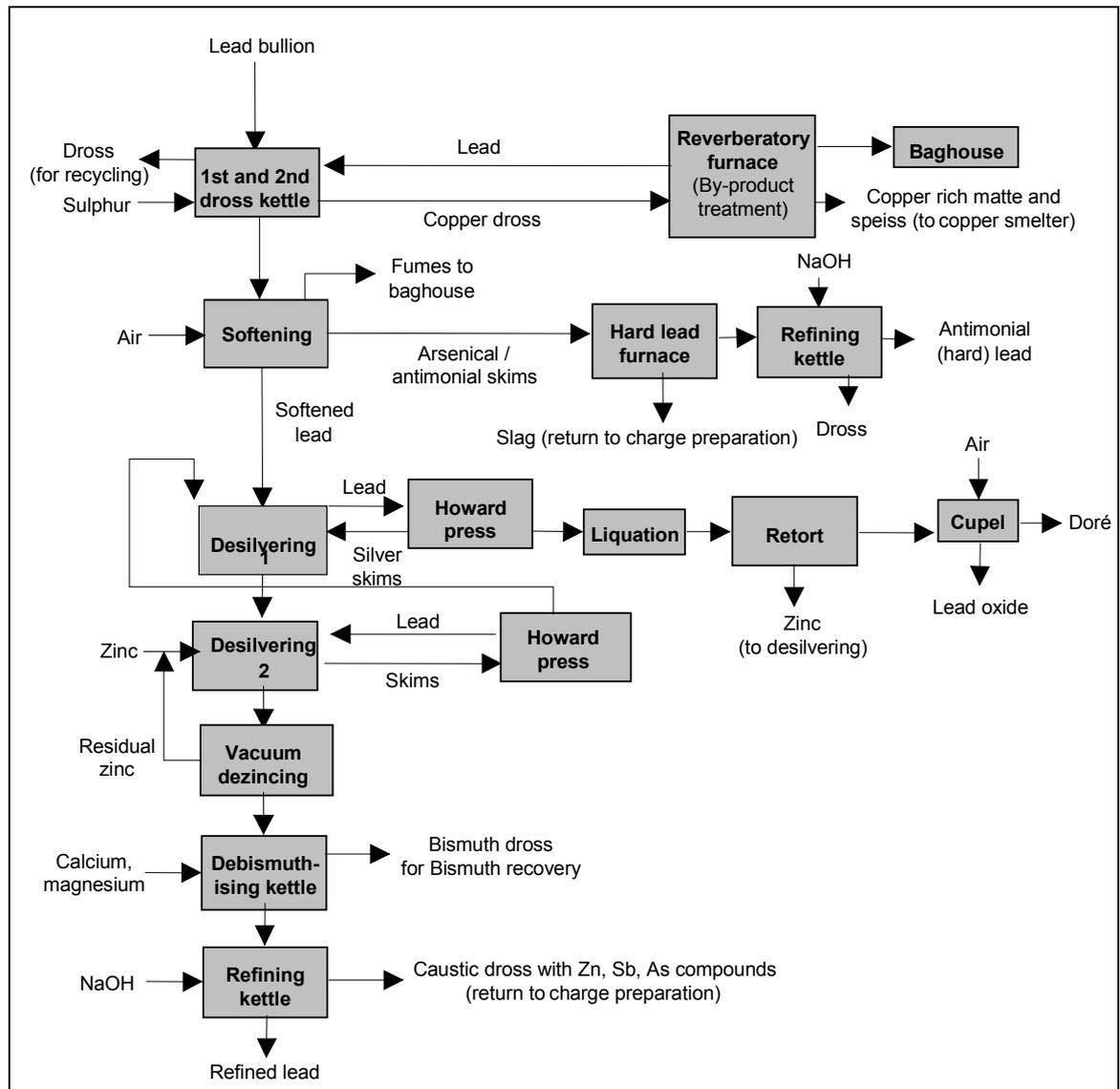
**Figure 5.3: Diagram of lead refining processes**
