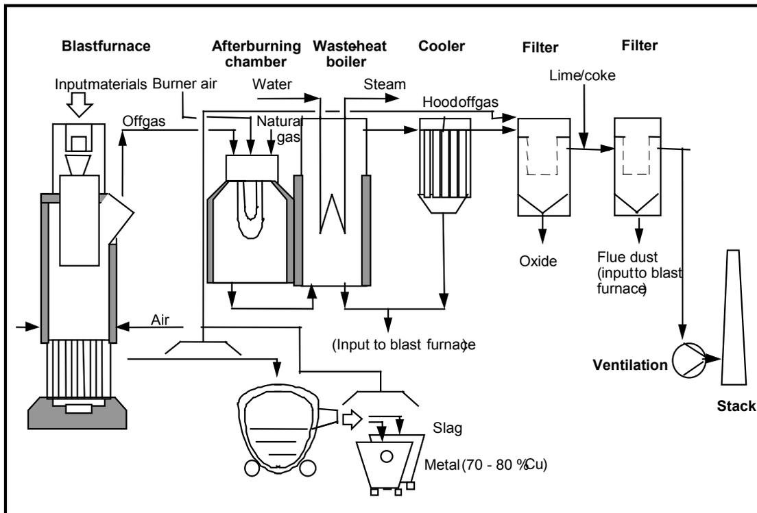
**Figure 2.5: Blast furnace for secondary copper production**
