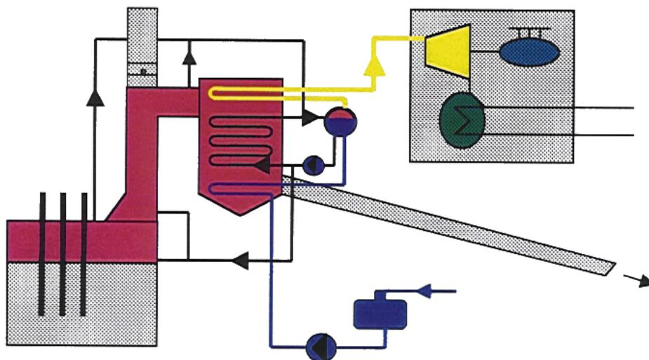
Figure 9.19: Energy recovery from a semi-closed furnace
