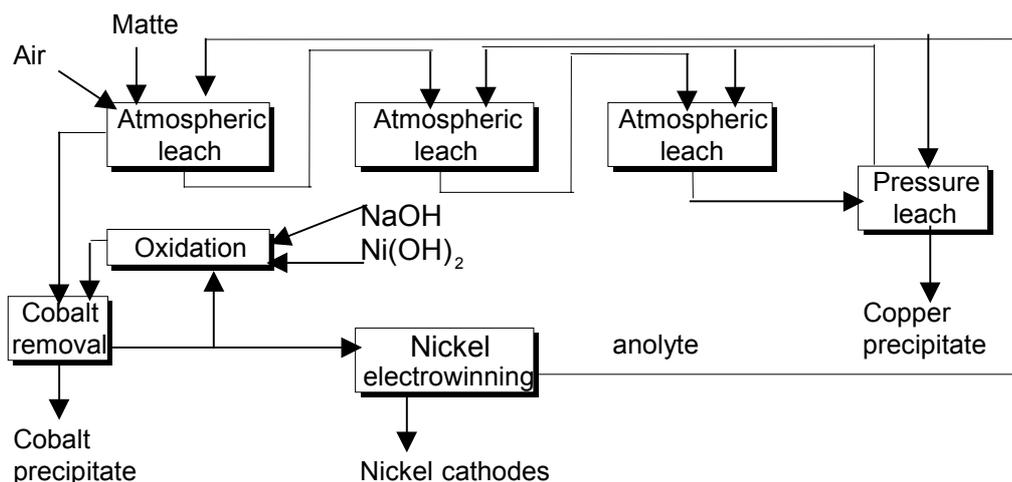
Figure 11.7: Sulphate based leaching process
