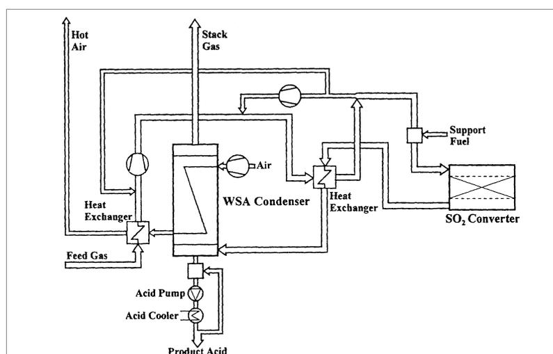
The catalyst used in the WSA technology is a potassium and sodium promoted vanadium catalyst in 10 and 20 mm extruded rings.
