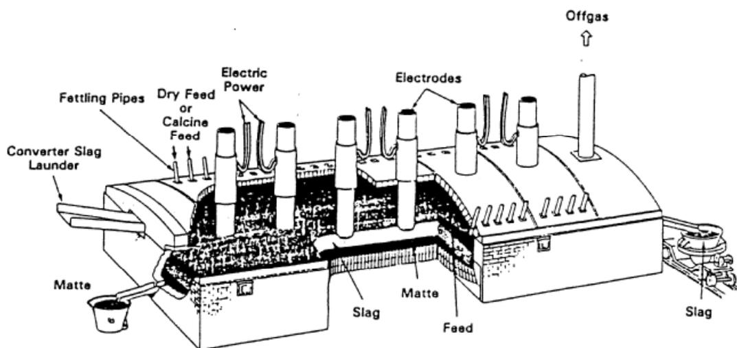
**Figure 2.8: Electric Furnace for concentrate or calcine smelting**
