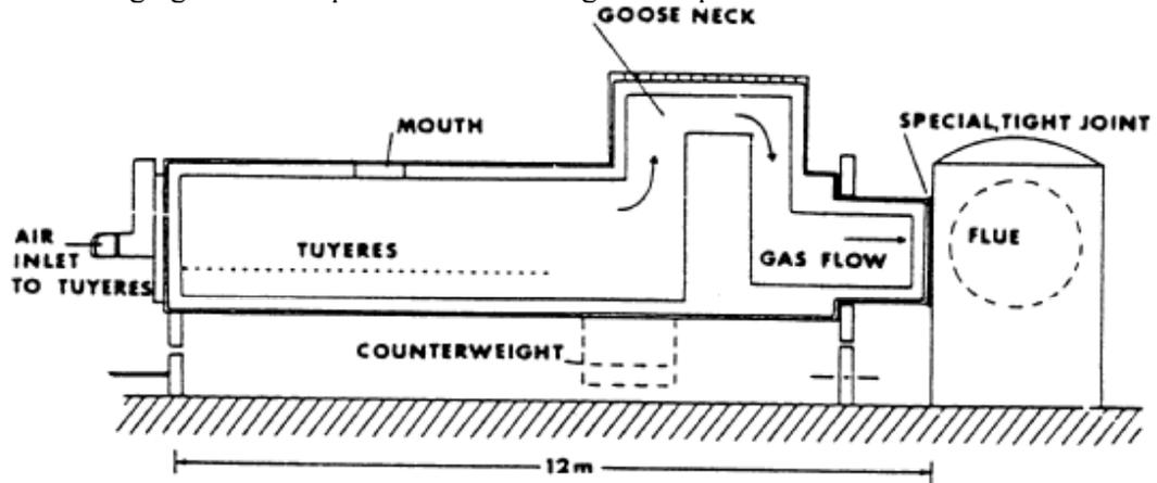
Figure 2.20: The Hoboken Converter
