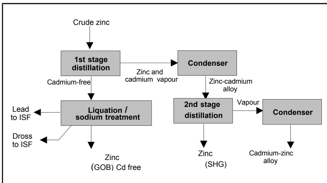
**Figure 5.4: Diagram of zinc/cadmium distillation**
