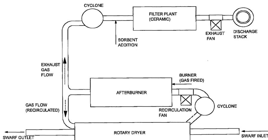
Figure 9.14: Gas cleaning system for a de-greasing plant
