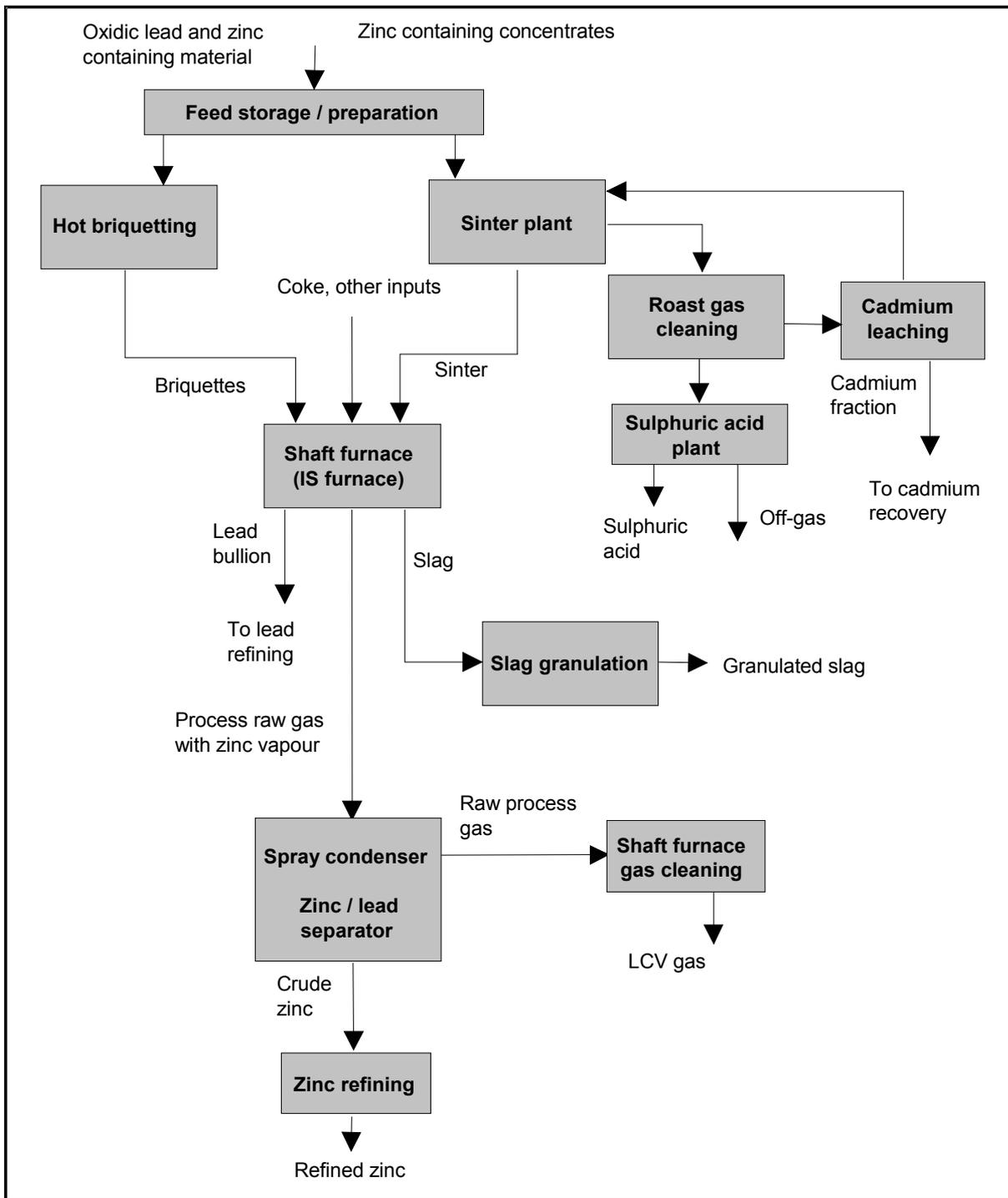
**Figure 5.1: Diagram of a typical Imperial Smelting Process for zinc and lead production [tm 102, DFIU Zn 1999]**
