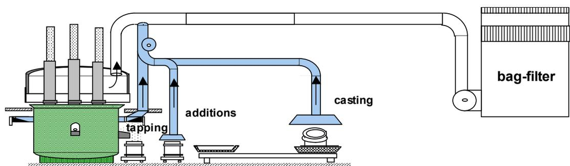
Figure 9.16: Collection of tapping and casting fume
