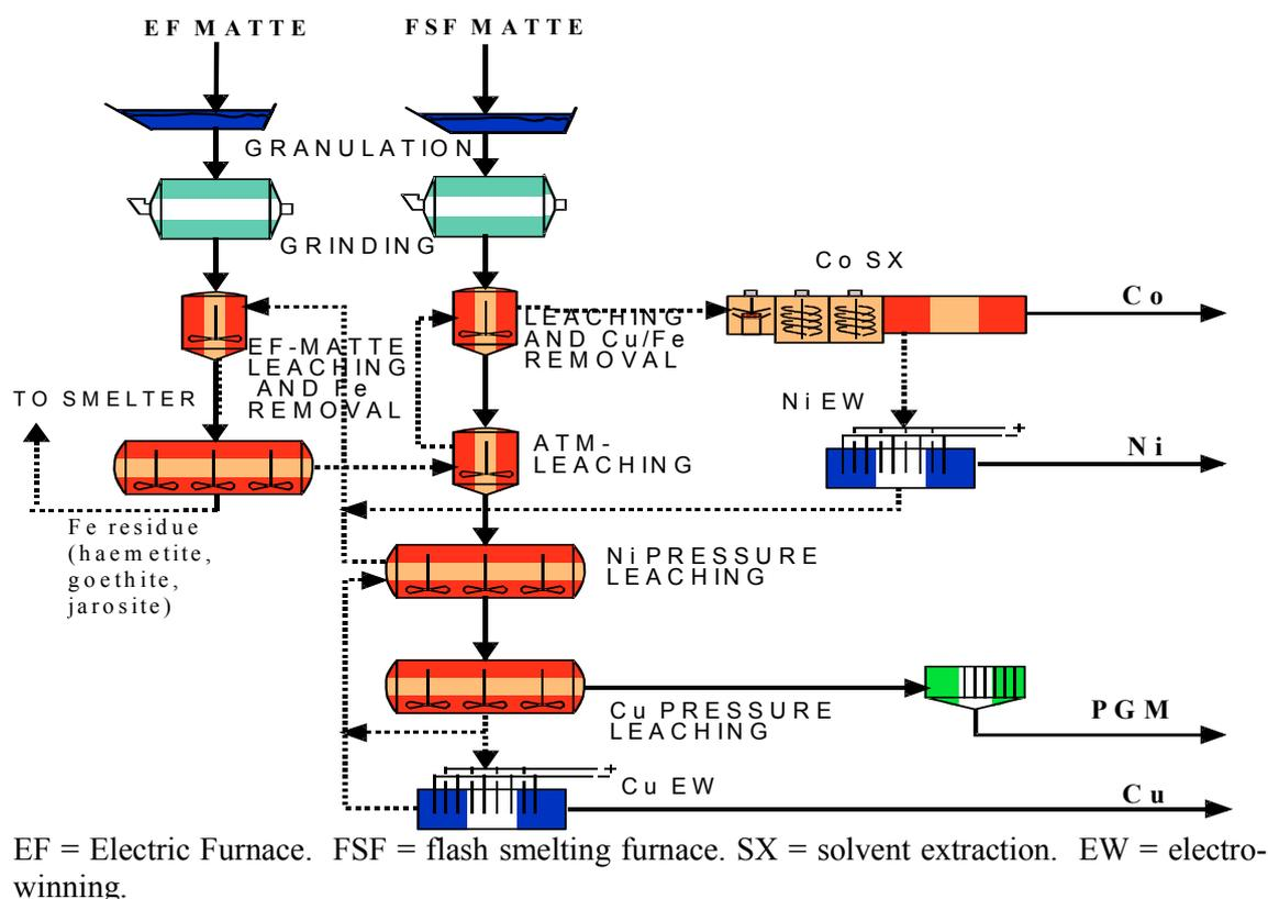
Figure 11.8: Flow sheet of the DON refinery process
