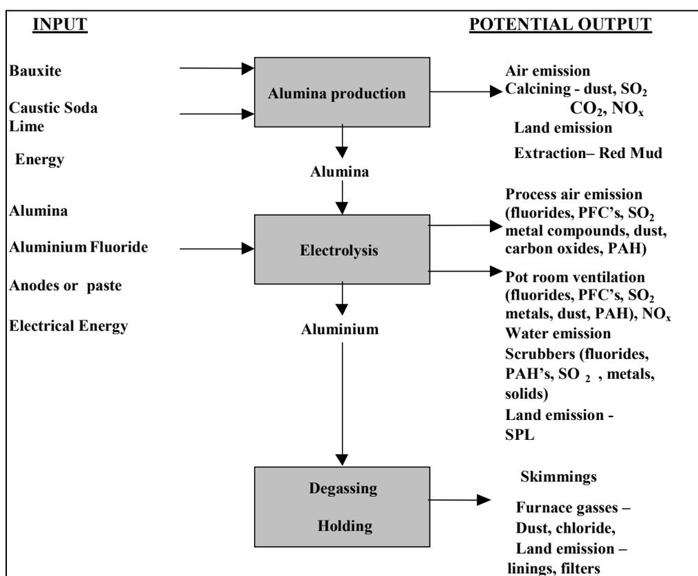
Figure 4.4: Input and output from primary aluminium production
