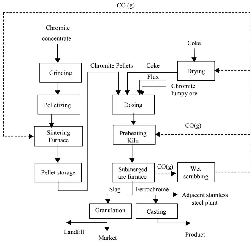
Figure 9.1: High-carbon ferro-chrome production by using a closed furnace
