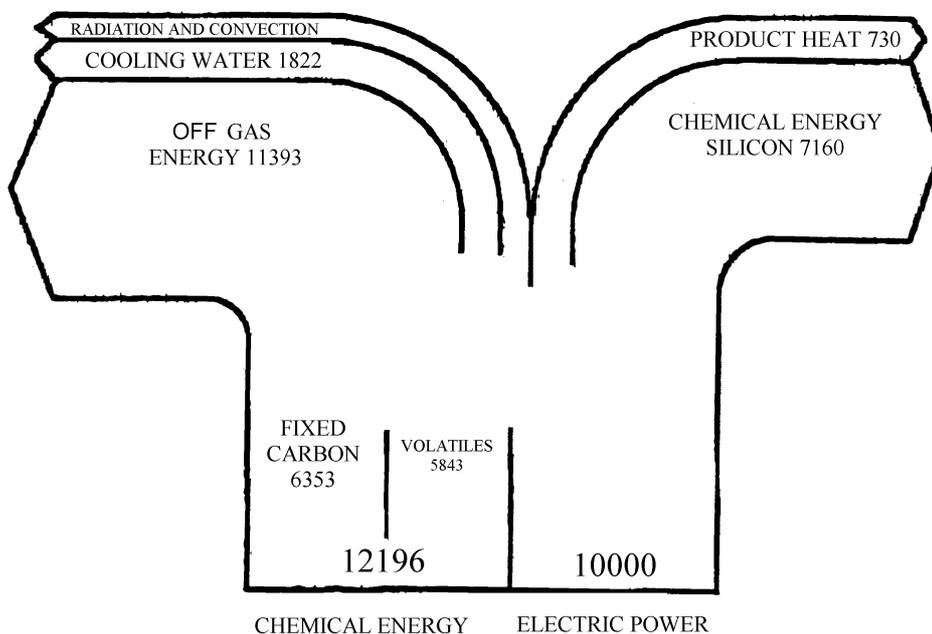
**Figure 9.13: Energy flow in a 10 MW silicon furnace**
