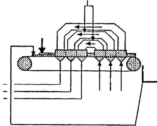
**Figure 2.3: Steel belt sintering furnace**
