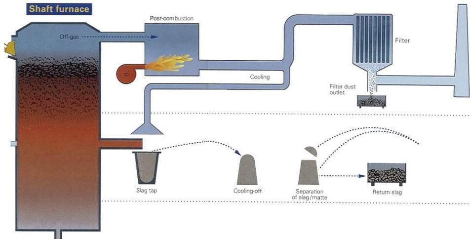
**Figure 5.10: Afterburner system used with a whole battery smelter**
